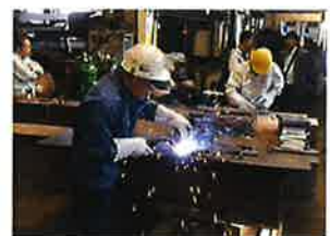
④仮組立て
